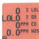
Red display in alarm conditions
