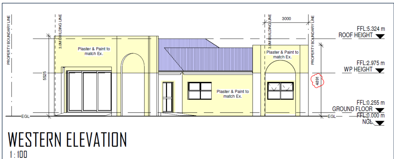
Figure 15: New height of 4.891m exceeding the regulatory 4m within 3m of the common boundary
