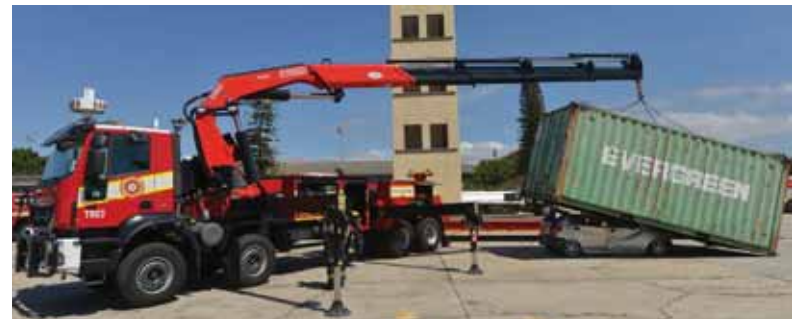
Heavy lifting: The Fire and Rescue Service's new R7,7 million Iveco Trakker 8x4 heavy-duty rescue recovery vehicle has a Fassi F660 crane with a lift capacity of 56,8 m and a maximum reach of 30,4 m. It also has two Waldon 30-ton hydraulic winches, each with a 60 m cable.
