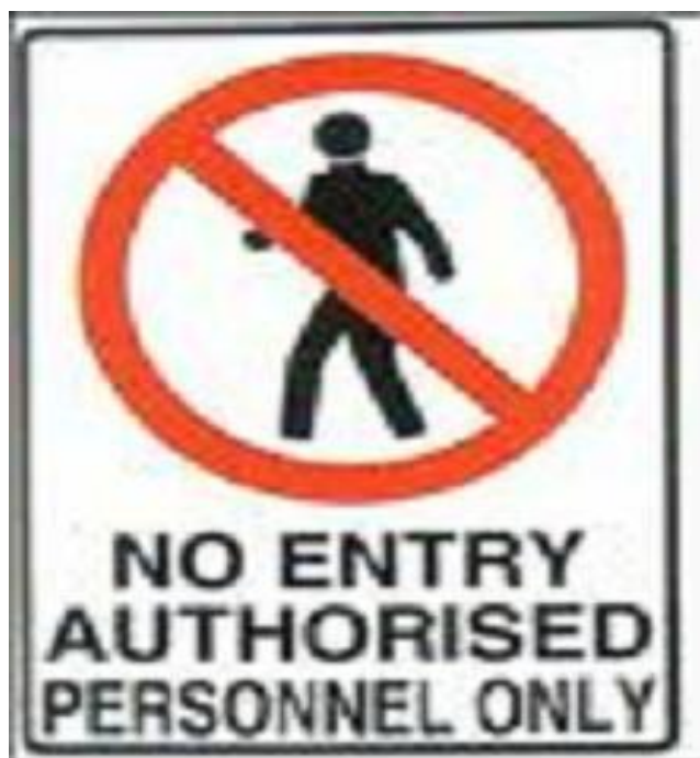
Figure F1: Unauthorized Entry Sign (Type PV3 to SANS 1186-1)
